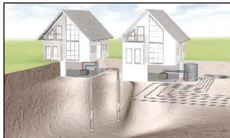
Figure 1. Vertical and horizontal loop (Source Rehau)
